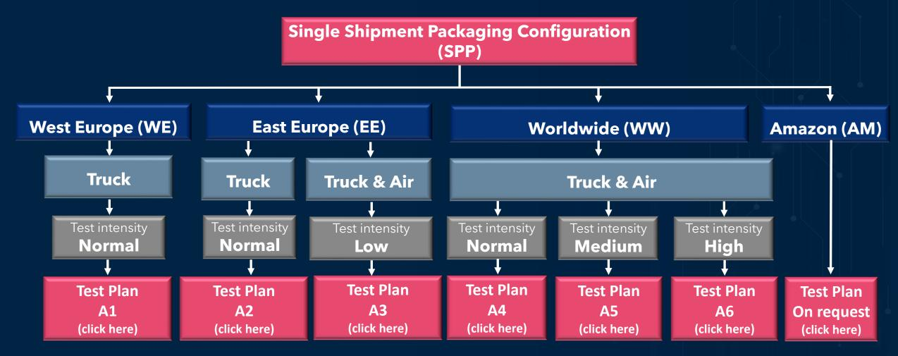
The measured vibration accelerations of a boat and train is not higher than 0,9 g-peak. The truck simulation on medium level is the acceleration >1,5g peak. In this case the truck simulation overrule the boat acceleration values.
